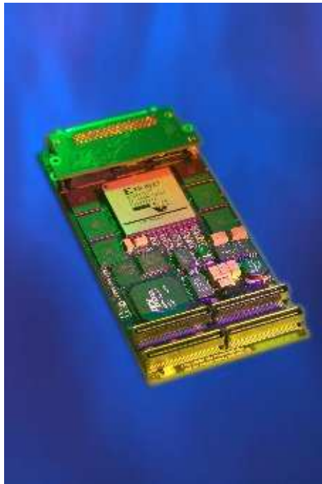
Xilinx Virtex-II Pro (XC2VP30) FPGA with 30,000 Logic Cells
